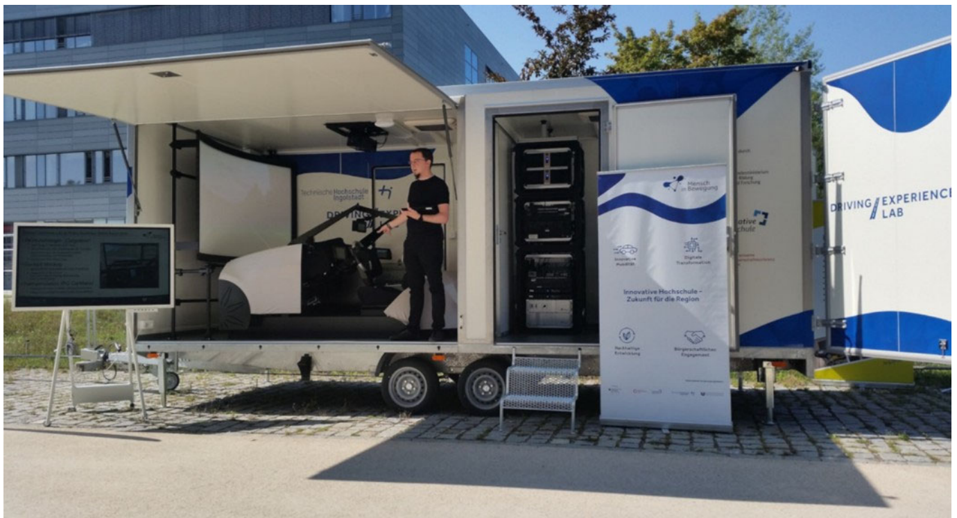
Figure 1: Overview of the Driving Experience Lab, left – mockup with open hatch, right – control room with a server rack.
