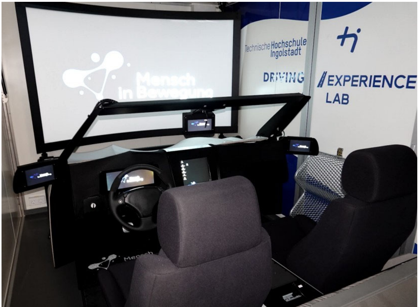
Figure 2: Vehicle cockpit mockup of DEL driving simulator room with visualization.
