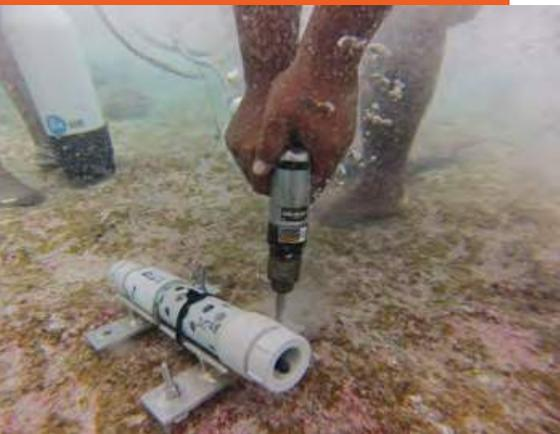
Deploying a pressure sensor on Fatato reef, Funafuti, Tuvalu. The data is analysed to extract short wave and infragravity wave information in order to gain insight on wave transformation on reef-fronted islands (April 2013).
