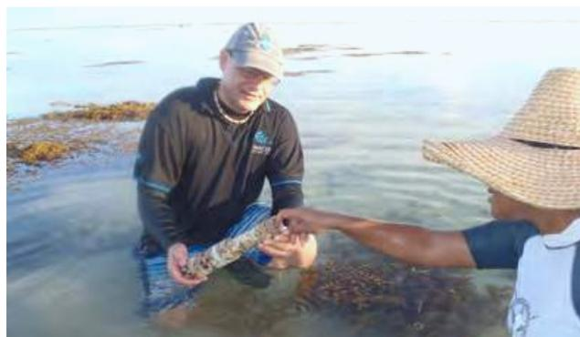
Recovering instruments that collected waves and water level data in Maui Bay, Fiji. The data was used to better understand coastal inundation on fringing coral reef and to better design inundation prediction tools (2014).
