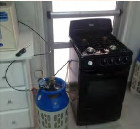
Modified stove with specialised H<sub>2</sub> gas burners connected to a low pressure gas storage cylinder and PEM electrolyser powered by a PV system (June 2015).
