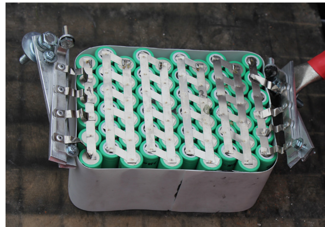
Short circuit test THI
